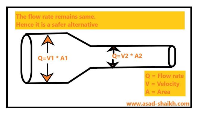
We know the Flow (Input from process engineer) and the Area (area of pipe is already known) and Hence Velocity can be easily calculated.
