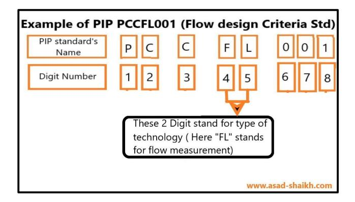
For level measurement the 4<sup>th</sup> & 5<sup>th</sup> digits are "LI"
